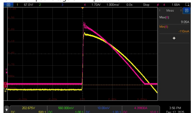
INPUT=230VAC/50HZ @ FULL LOAD CH1: AC Input Voltage CH4: Input current
