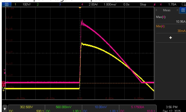
INPUT=277VAC/50HZ @ FULL LOAD CH1: AC Input Voltage CH4: Input current
