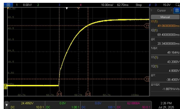
INPUT=115VAC/60HZ @ FULL LOAD CH1: Output Voltage
