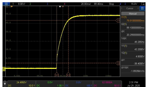
INPUT=230VAC/50HZ @ FULL LOAD CH1: Output Voltage
