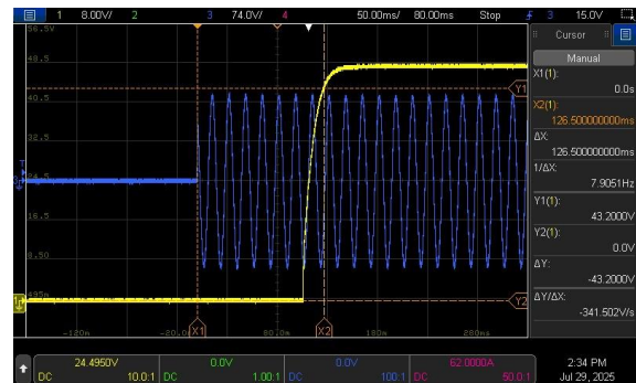
INPUT=115VAC/60HZ @ FULL LOAD CH1: Output Voltage CH3: AC Input Voltage
